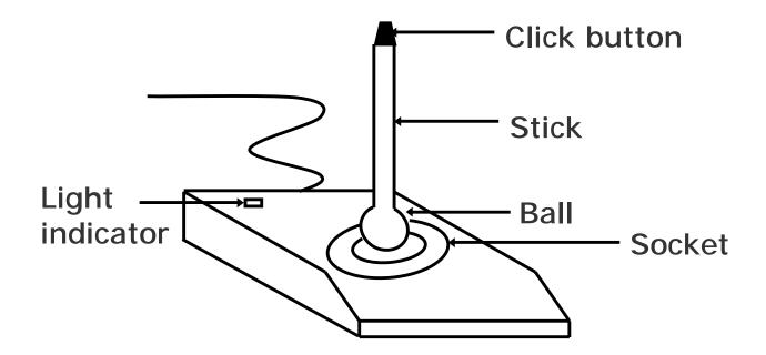
Commonly used for video games, flight simulators, training simulators, and for controlling industrial robots
